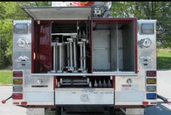
Low ground ladder storage with safe and easy access to hose and equipment
